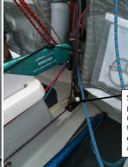
Single block and tie off point for control line on mast step. Providing turning point to centreboard case cleat and flip-flop block.
