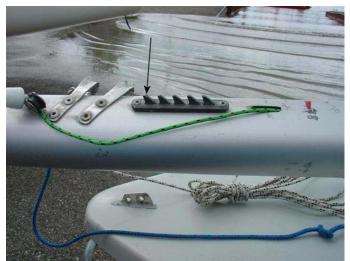
Solution No2, Tooth rack for wire halyards only. If you use the last tooth (as shown by the arrow) or if there is only one, it is as good as a stopper, since you have only one possible position for the mainsail. If the correct position for the halyard is the middle one for example, you must cut out the remaining teeth, or use solution No3 below.
