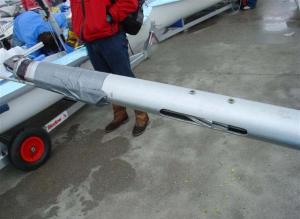
Solution No1, Mast head lock. Those who have this kind of fitting installed don't need a separate stopper since this arrangement only permits a single position for the mainsail. Just make sure your sail fits exactly within the limits!
