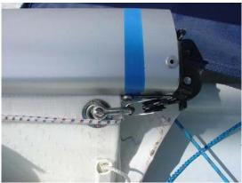
In this example of a boom stopper, the rivet has been installed a few mm inside the limit. You may also cut the boom spar so the end fitting is at the limit point itself, as in the following picture:
