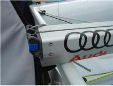
NOTE THAT IF YOU MODIFY THE STANDARD ISSUE LIMIT MARKS (AS PROVIDED BY THE MAST MANUFACTURERS) YOU MUST PUT NEW ONES MADE OF PERMANENT TAPE OR PAINT (SEE THE RULES FOR MORE DETAILS, INCLUDING THE DEFINITION OF A PERMANENT TAPE).
