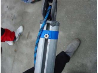
Solution No3, Rivet (pictured) or screw in the sail track. In this example, the stopper is positioned for mainsails with square-cut boltrope at the head. In the following picture, you see that if you change into a mainsail with cut-down boltrope, then the stopper for a normal mainsail will not work anymore:
